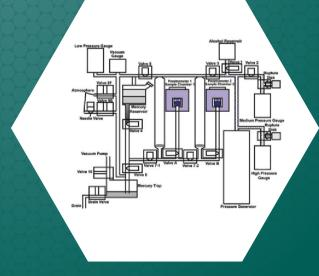
The cell is closed with a lid and placed in the sample chamber. Intrusion volume of mercury is measured by noting changes in mercury level in the penetrometer with a magnetic sensor. Exposure to mercury is negligible due to the unique design of the instrument. The unique design also permits use of nonmercury nonwetting liquids for intrusion. Another instrument design uses water as the nonwetting liquid and uses absolutely no mercury. The instrument is known as the Aquapore.
